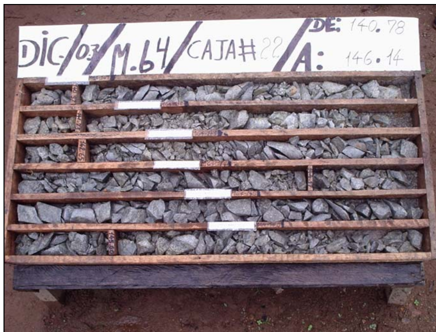
Figure 7.2 Drill Core Photo of DDH M64 Showing Low RQD
