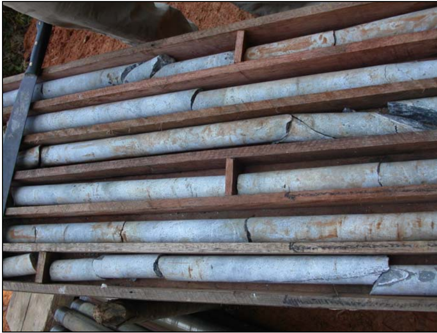
Figure 7.3 Drill Core with Unaltered Anhydrite (Below the Gypsum Front)
